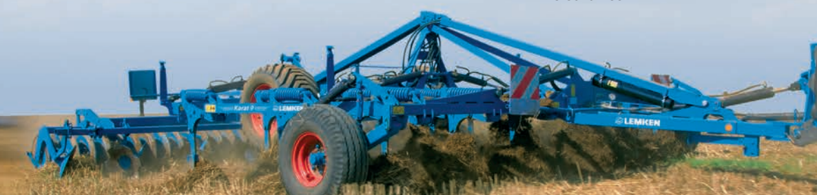
11" (28 cm) line distance, 28" or 39" (71 cm or 99 cm) beam spacing, 31" (79 cm) underframe clearance
