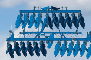
5" (12.5 cm) line distance, 42" or 47" (107 or 120 cm) beam spacing
