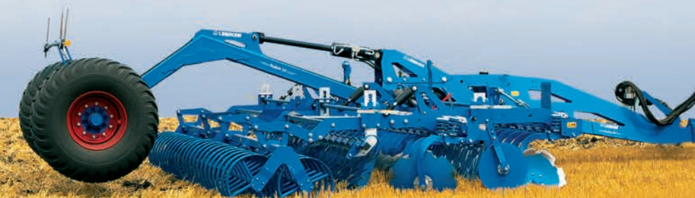
20° cutting angle to the ground; 17° to the direction of travel for the first row of discs and 15° for the second
