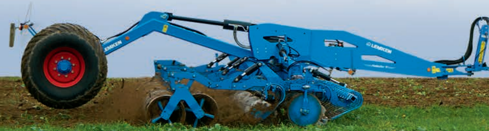
Dual disc angle of 10.5° to the soil and 16.5° to the direction of travel
